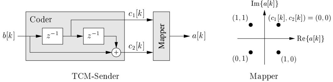
The convolutional encoder uses the data bits  $b[k]$  to produce two code bits at each step,  $c_1[k] = b[k-1]$  and  $c_2[k] = b[k] \oplus b[k-2]$  ( $\oplus$  denotes addition modulo 2). The symbol mapper maps these code bits to symbols  $a[k]$  (with  $|a[k]|^2 = 2$ ).
