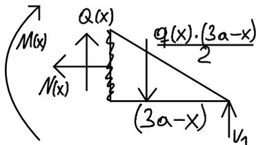
$$\frac{q_0}{a} = \frac{q(x)}{(3a-x)} \rightarrow q(x) = \frac{q_0}{a} (3a-x)$$
