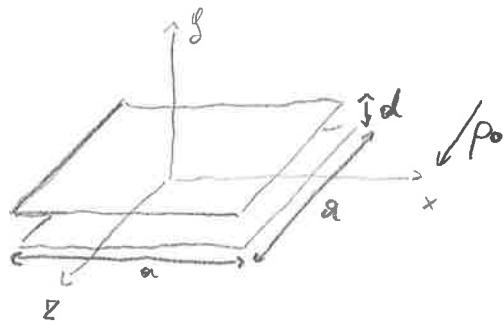
$$\Phi(x, y, z, t) = -\frac{t}{\gamma} E_0 y$$
