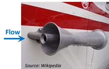
Venturi tube on the hull of an airplane for velocity measurements
