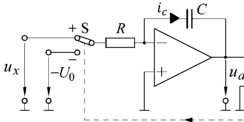
$$u_c = \frac{1}{C} \int_{t_1}^{t_2} i_c dt$$
