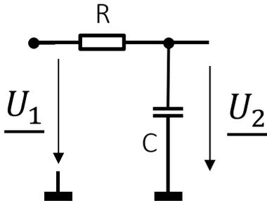
$$G(j\omega) = \frac{U_2}{U_1} = \frac{1/j\omega C}{R + 1/j\omega C} = \frac{1}{1 + j\omega \underbrace{RC}_{\tau}}$$
