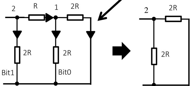
$$\Rightarrow i_0 = \frac{i_1}{2}, i_1 = \frac{i_2}{2}, \dots, i_5 = \frac{i_{ges}}{2}$$
