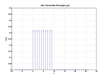
The triangle of overall length 19 requires the convolution of a rectangle of overall duration 10 with itself, which cannot be centered in time-domain, since there is *no central element*. However, the convolution can be calculated for a rectangle spanning 0...9 and shifting the triangle in *frequency domain*:
