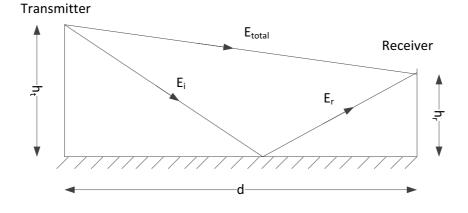
Figure 1: Two-ray ground reflection model
