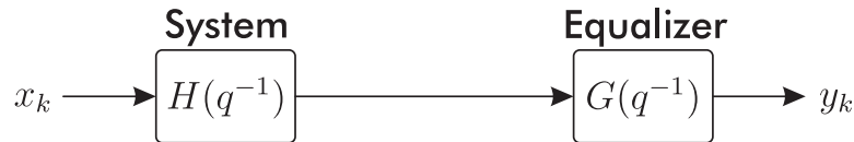
Figure 1.3: Basic setup of linear system and its equalizer.
